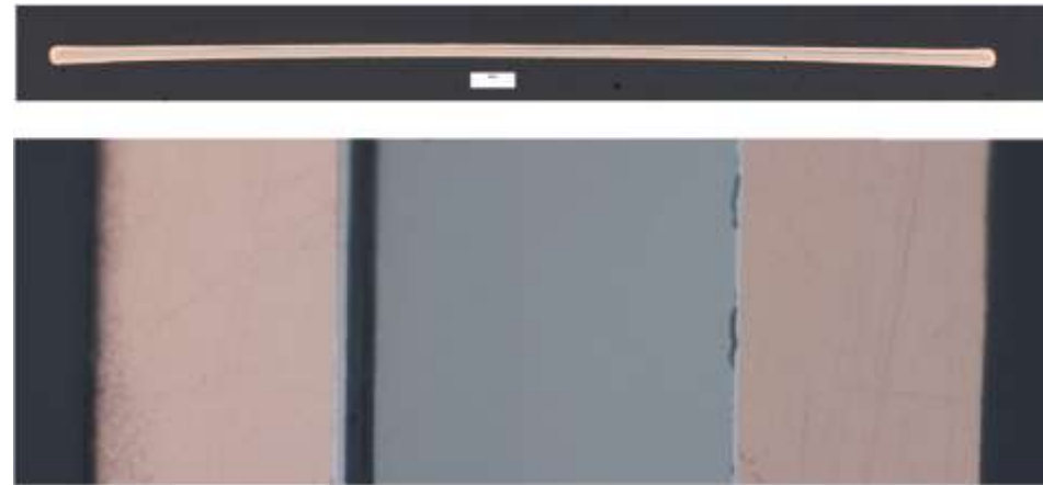
Cu-plated HTS conductor, 45 \mu m single Cu-layer
