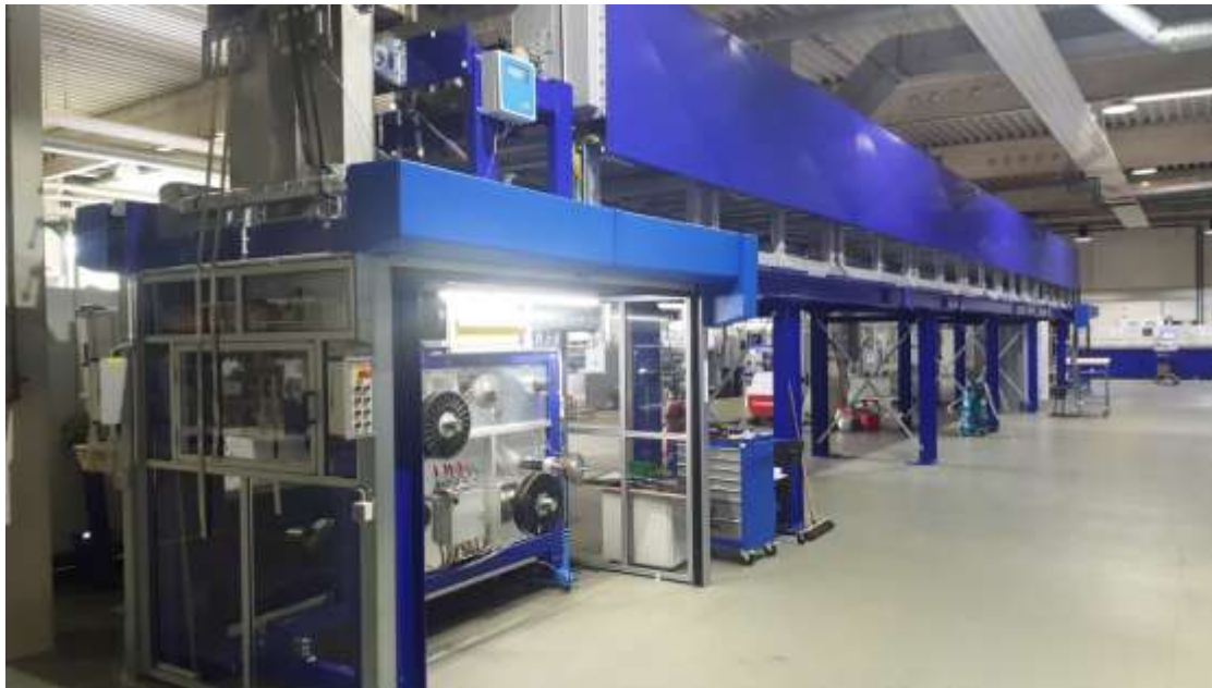
4x25m high temperature annealing furnace
