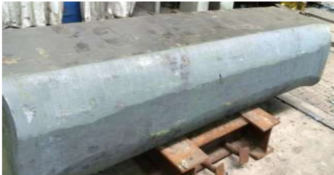
~10 t ingot processed to 60 μ tape
